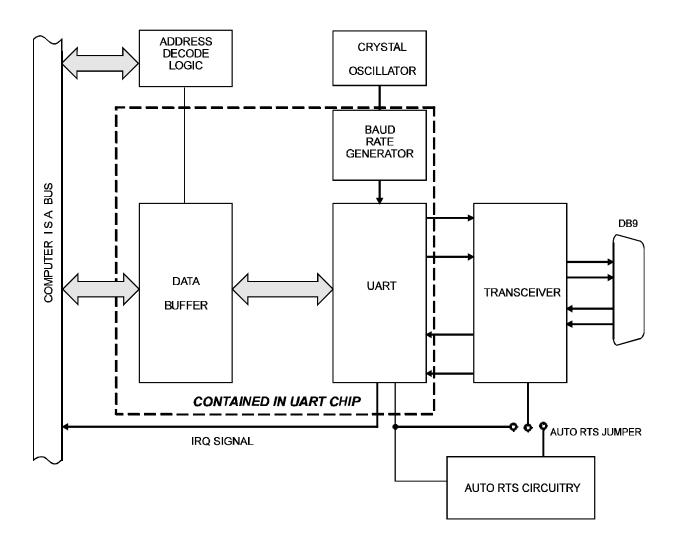
**Figure 1-1:** COM-2S Block Diagram (Only one serial channel shown)
