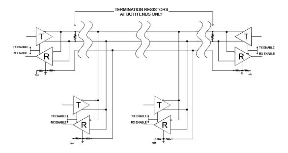
Figure A-1: Typical RS485 Two-Wire Multidrop Network
