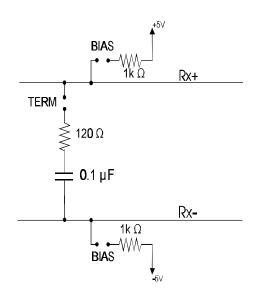
Figure 3-1: Simplified Termination Schematic
