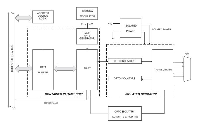
Figure 1-1: ICOM422/485A Block Diagram
