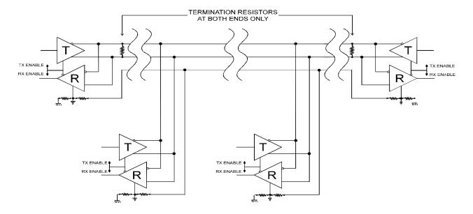
Figure A-1: Typical RS485 Two-Wire Multidrop Network
