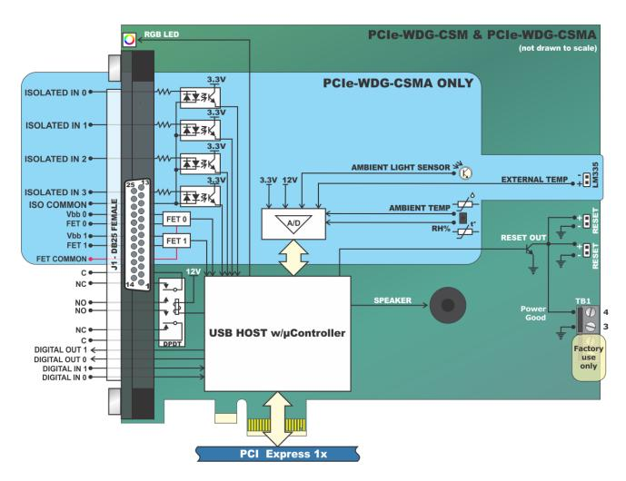
Figure 1-1: Block Diagram
